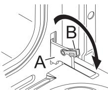
Grip the sides of the door and lift it upwards and slide it forward to remove. To refit the door, slide the hinges into their slots. Before closing the door, **remember to rotate the two toggles B,** used to lock the two hinges, fully back.
